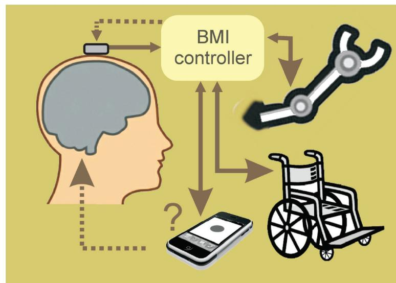
**Figure TF32-2:** The basic BMI loop depends on (a) neural recording, (b) a computational device or controller that maps neural signals to control signals to the prosthetics, and (c) feedback to the user or patient. Perhaps one day BMIs will even drive the use of portable consumer devices!
