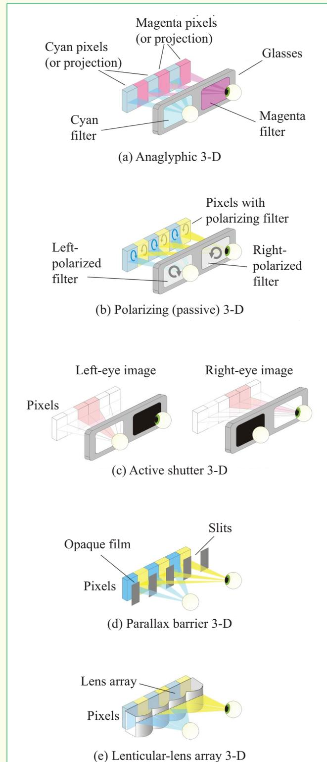
**Figure TF28-1:** Various techniques for realizing 3-D imaging.
