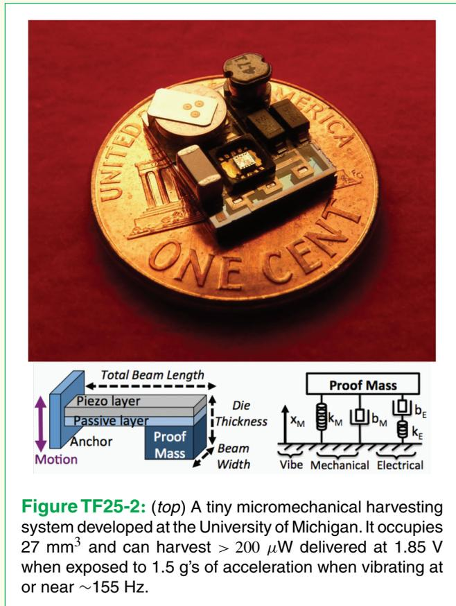
**Figure TF25-2:** (top) A tiny micromechanical harvesting system developed at the University of Michigan. It occupies  $27 \text{ mm}^3$  and can harvest  $> 200 \mu\text{W}$  delivered at  $1.85 \text{ V}$  when exposed to  $1.5 \text{ g}$ 's of acceleration when vibrating at or near  $\sim 155 \text{ Hz}$ .
