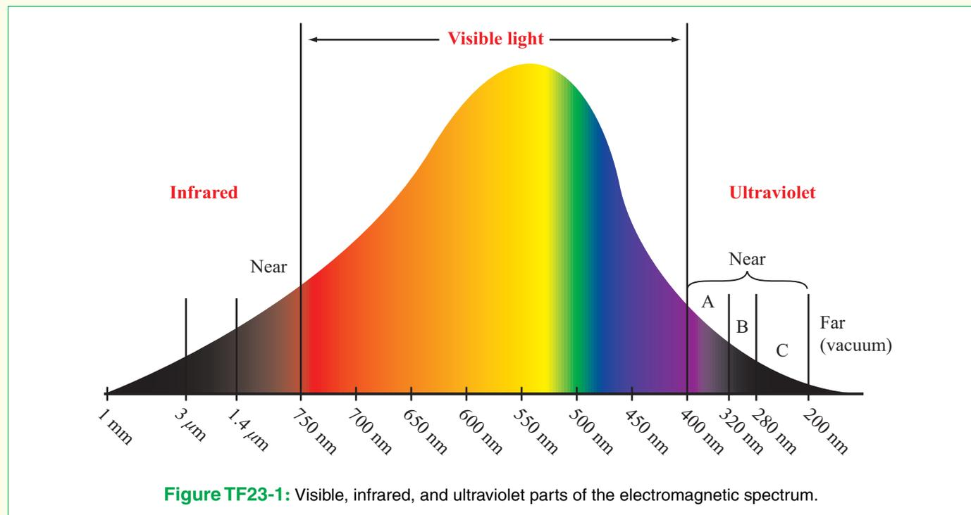
**Figure TF23-1:** Visible, infrared, and ultraviolet parts of the electromagnetic spectrum.
