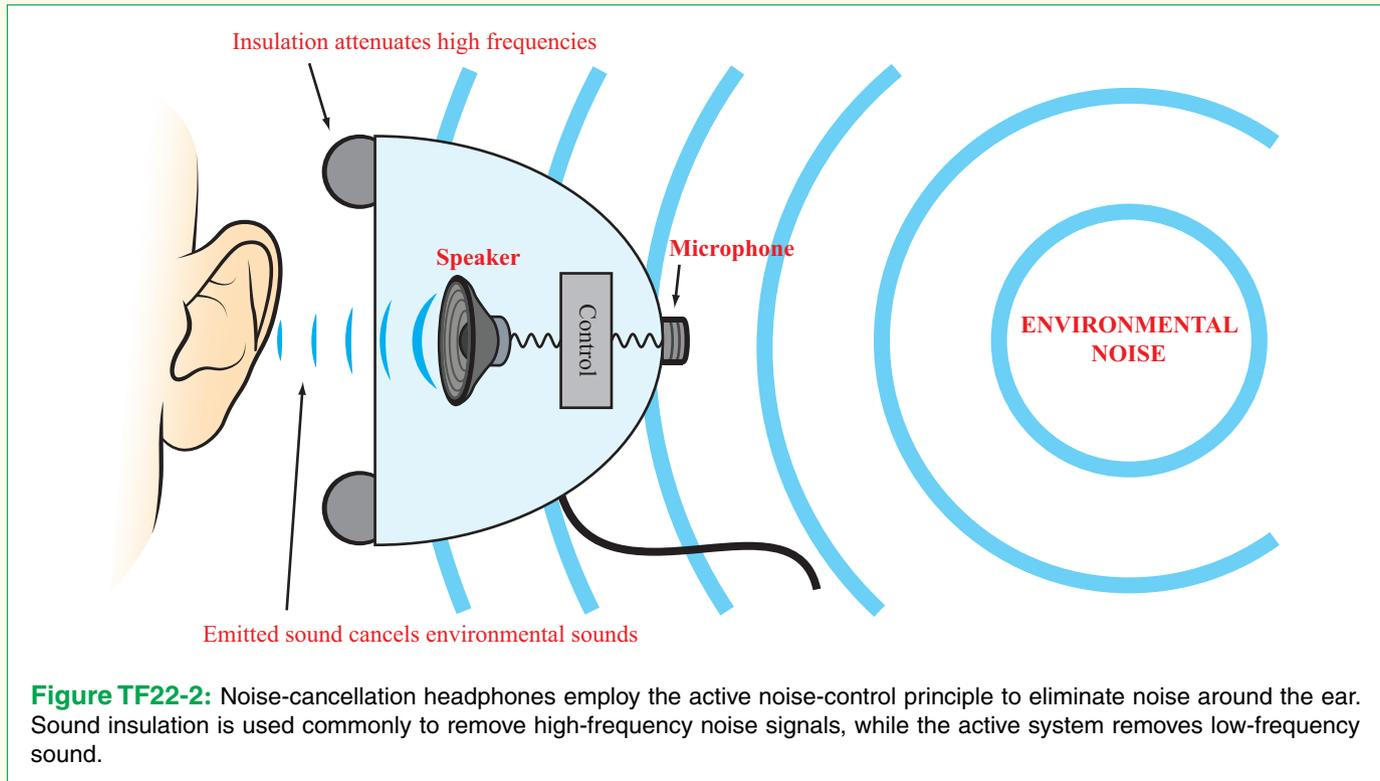
**Figure TF22-2:** Noise-cancellation headphones employ the active noise-control principle to eliminate noise around the ear. Sound insulation is used commonly to remove high-frequency noise signals, while the active system removes low-frequency sound.
