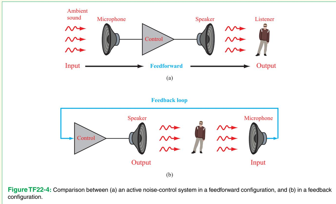
**Figure TF22-4:** Comparison between (a) an active noise-control system in a feedforward configuration, and (b) in a feedback configuration.
