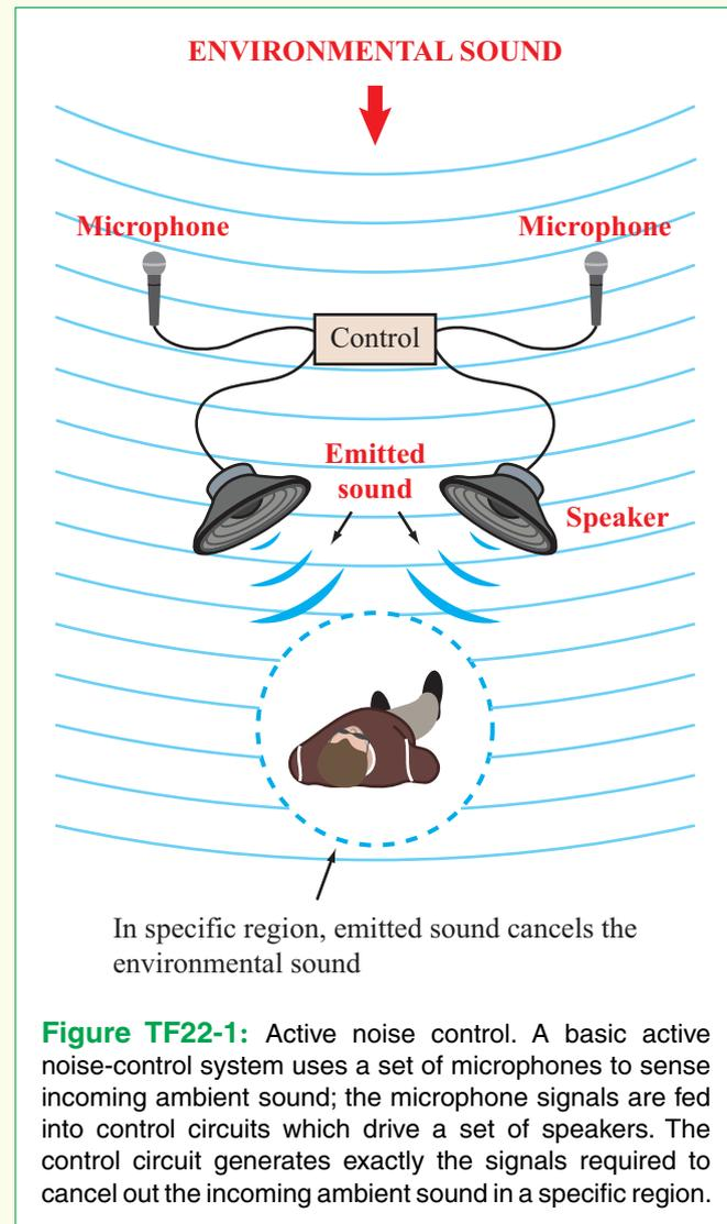
**Figure TF22-1:** Active noise control. A basic active noise-control system uses a set of microphones to sense incoming ambient sound; the microphone signals are fed into control circuits which drive a set of speakers. The control circuit generates exactly the signals required to cancel out the incoming ambient sound in a specific region.
