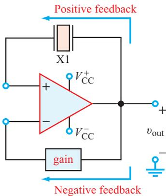
**Figure TF19-2:** Schematic block diagram of an oscillator circuit. An oscillator is wired into the positive feedback path, while a negative feedback path is used to control gain.
