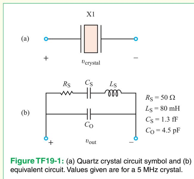
**Figure TF19-1:** (a) Quartz crystal circuit symbol and (b) equivalent circuit. Values given are for a 5 MHz crystal.
