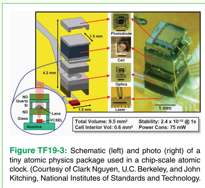
**Figure TF19-3:** Schematic (left) and photo (right) of a tiny atomic physics package used in a chip-scale atomic clock. (Courtesy of Clark Nguyen, U.C. Berkeley, and John Kitching, National Institutes of Standards and Technology.)
