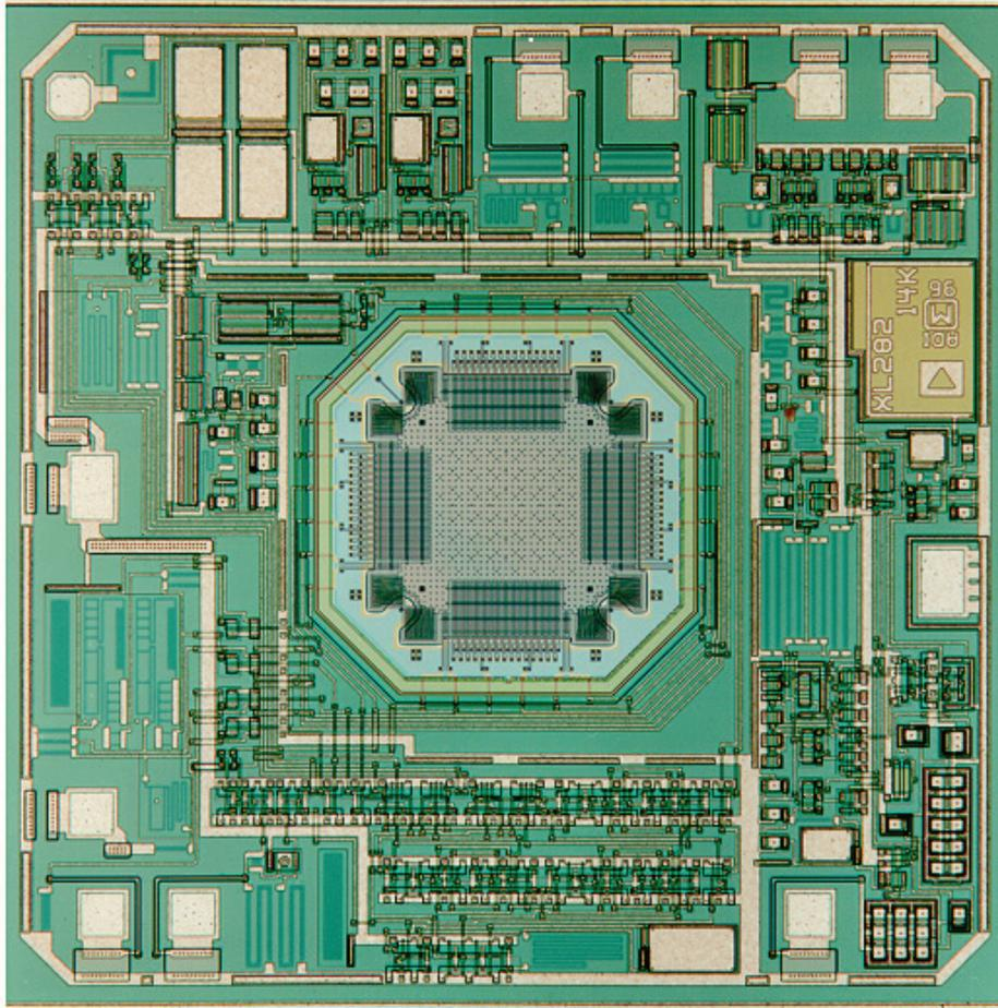
**Figure TF15-3:** The complete ADXL202 accelerometer chip. The center region holds the micromechanical sensor; the majority of the chip space is used for the electronic circuits that measure the capacitance change, provide feedback, convert the measurement into a digital signal, and perform self-tests. (Courtesy of Analog Devices.)
