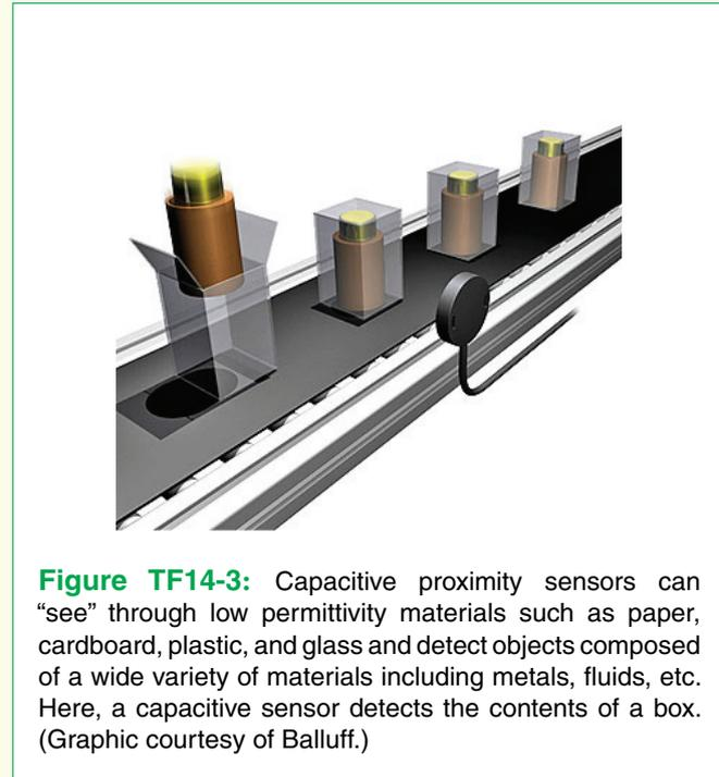
**Figure TF14-3:** Capacitive proximity sensors can “see” through low permittivity materials such as paper, cardboard, plastic, and glass and detect objects composed of a wide variety of materials including metals, fluids, etc. Here, a capacitive sensor detects the contents of a box. (Graphic courtesy of Balluff.)
