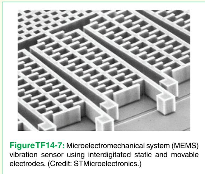
**Figure TF14-7:** Microelectromechanical system (MEMS) vibration sensor using interdigitated static and movable electrodes. (Credit: STMicroelectronics.)
