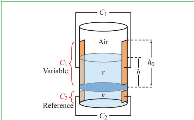
**Figure TF14-4:** Fluid height can be measured from the outside of a plastic or glass tank using a pair of parallel plate capacitors on the outside of the tank.
