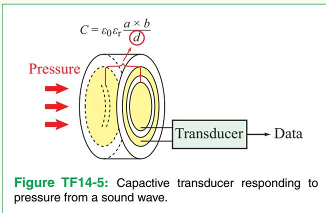
**Figure TF14-5:** Capacitive transducer responding to pressure from a sound wave.
