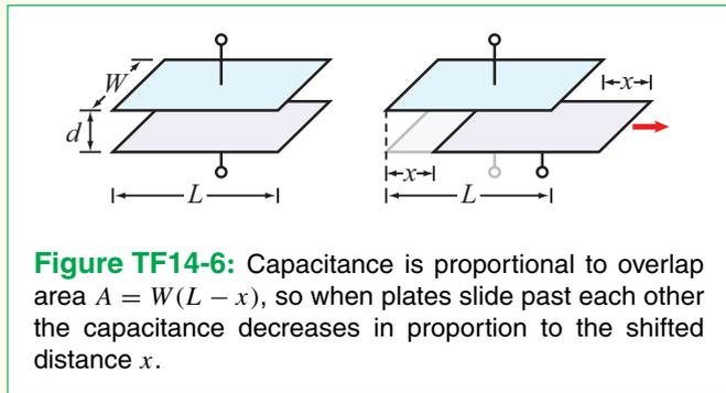
**Figure TF14-6:** Capacitance is proportional to overlap area  $A = W(L - x)$ , so when plates slide past each other the capacitance decreases in proportion to the shifted distance *x*.
