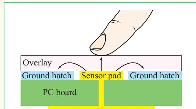
**Figure TF14-1:** A capacitive touch sensor uses the high permittivity of the finger to change the capacitance. The finger does not need to come in direct contact with the sensor in order to be detected.
