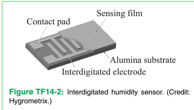
**Figure TF14-2:** Interdigitated humidity sensor. (Credit: Hygrometrix.)
