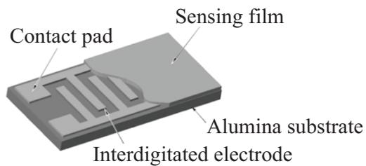
**Figure TF14-2:** Interdigitated humidity sensor. (Credit: Hygrometrix.)
