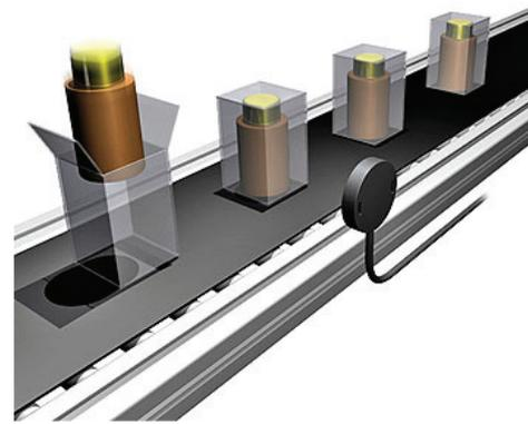
**Figure TF14-3:** Capacitive proximity sensors can “see” through low permittivity materials such as paper, cardboard, plastic, and glass and detect objects composed of a wide variety of materials including metals, fluids, etc. Here, a capacitive sensor detects the contents of a box. (Graphic courtesy of Balluff.)
