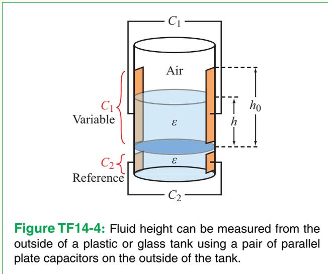
**Figure TF14-4:** Fluid height can be measured from the outside of a plastic or glass tank using a pair of parallel plate capacitors on the outside of the tank.
