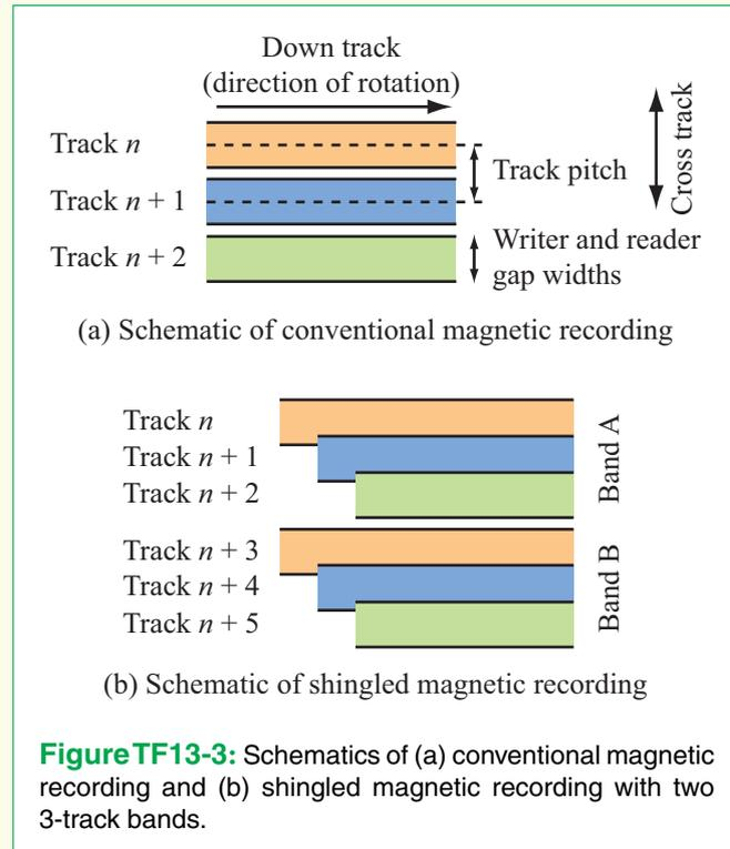
**Figure TF13-3:** Schematics of (a) conventional magnetic recording and (b) shingled magnetic recording with two 3-track bands.
