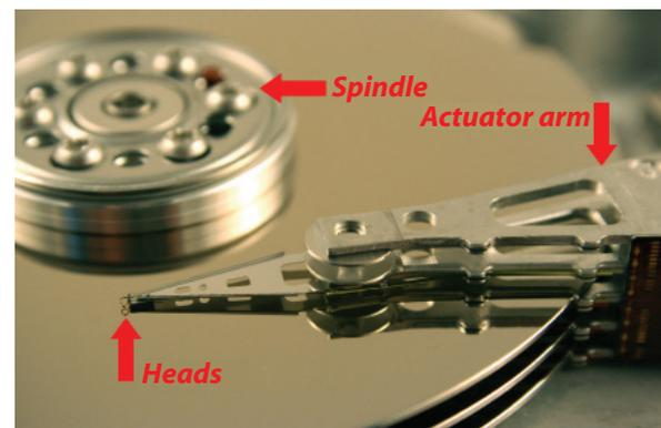
**Figure TF13-2:** Close-up of a disassembled hard drive showing the magnetic discs mounted on a spindle and an actuator arm. The head sits at the end of the arm and performs the read/write operations as the disc spins.
