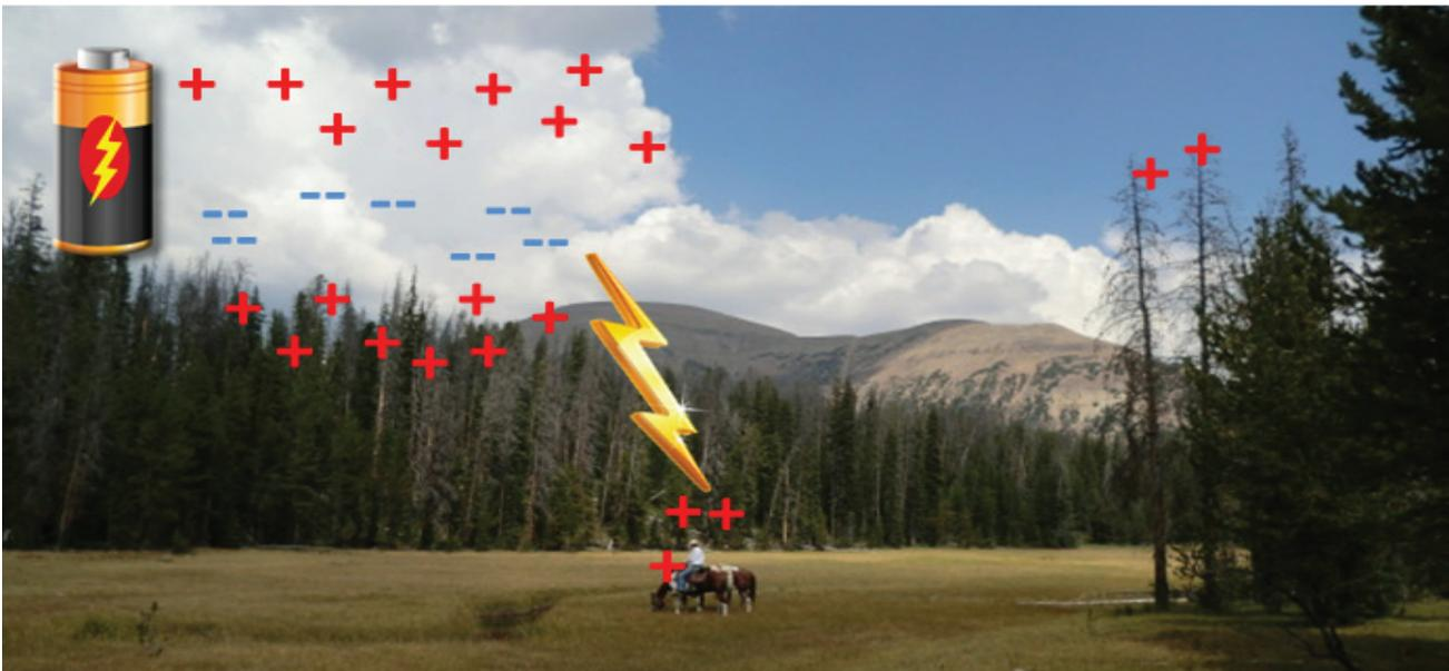
**Figure TF2-1:** Turbulent air causes negative charges to build up on the bottom of cumulonimbus clouds, separated from the positive charges on the top. The negative charges attract positive charges from the Earth, which move to the top of tall objects. A lightning strike can occur between the negative cloud and positive Earth charges.
