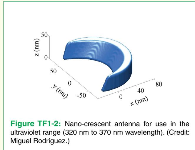
**Figure TF1-2:** Nano-crescent antenna for use in the ultraviolet range (320 nm to 370 nm wavelength). (Credit: Miguel Rodriguez.)
